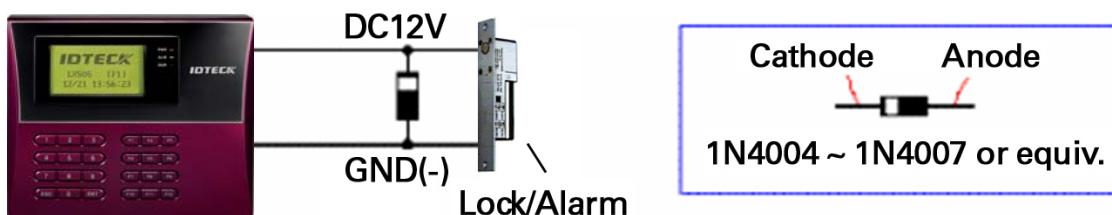
Figure: Reverse Diode Connection
