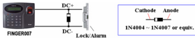
Figure : Reverse Diode connection
